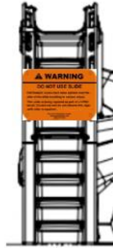
Sign in the correct location
